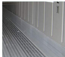
The inner scufflining makes the lining less prone to impacts and reduces the need for repair inside the reefer.
